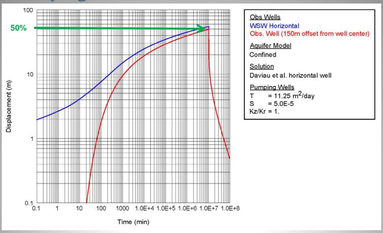
After iteration, 20 years of pumping at 620 m<sup>3</sup>/d yields 50% drawdown at radius of 150 m
