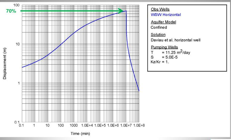
After iteration, 20 years of pumping at 800m<sup>3</sup>/d yields 70% drawdown at pumping well
