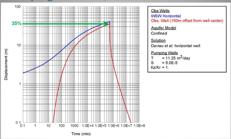
After iteration, 1 year of pumping at 600 m<sup>3</sup>/d yields 35% drawdown at radius of 150 m
