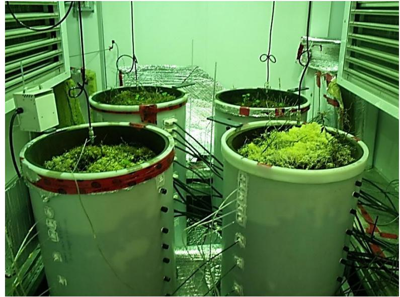
**29 TDR probes for soil moisture measurements,
