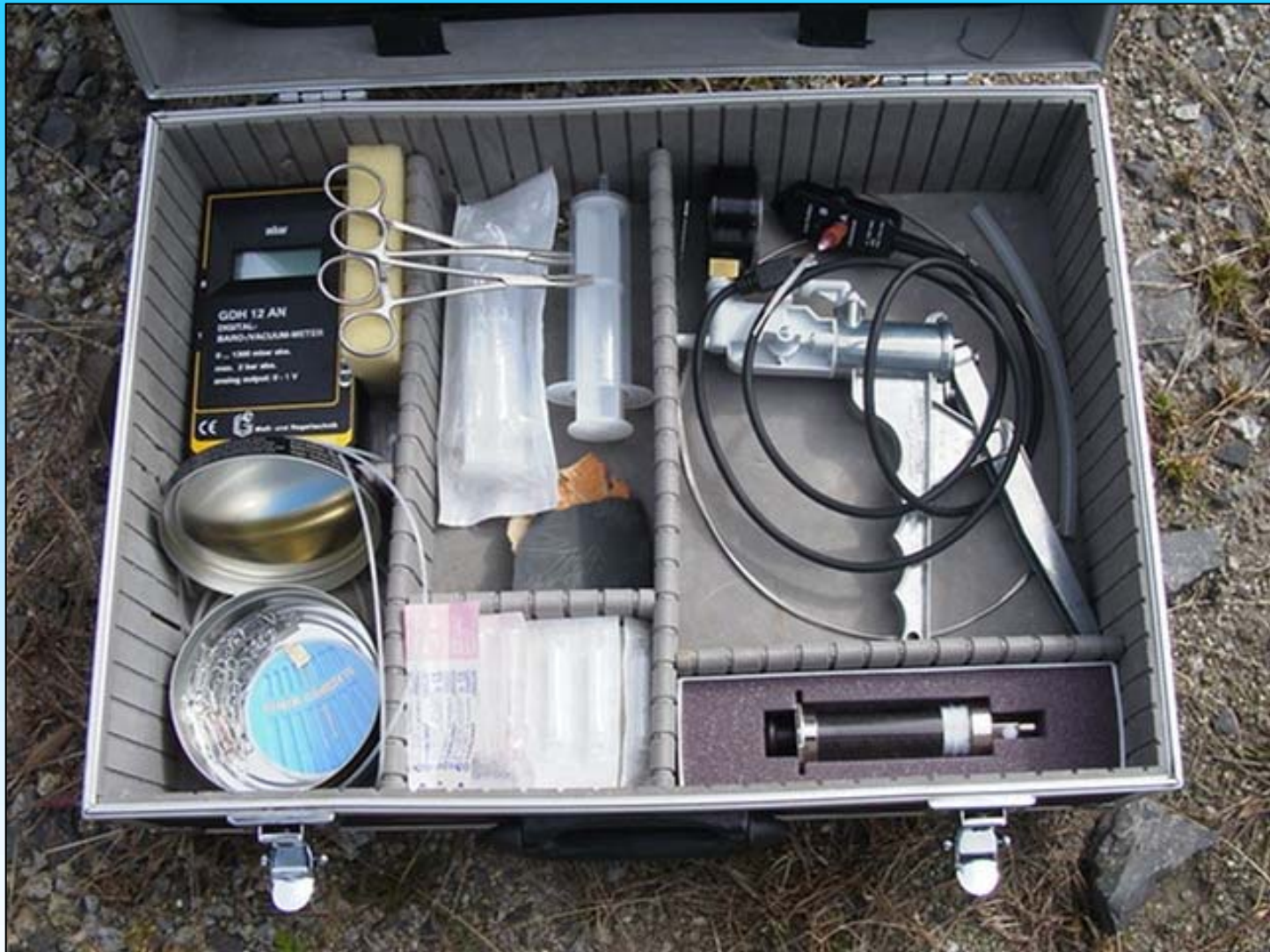
Sampling set to collect gas samples from GASSYS.
