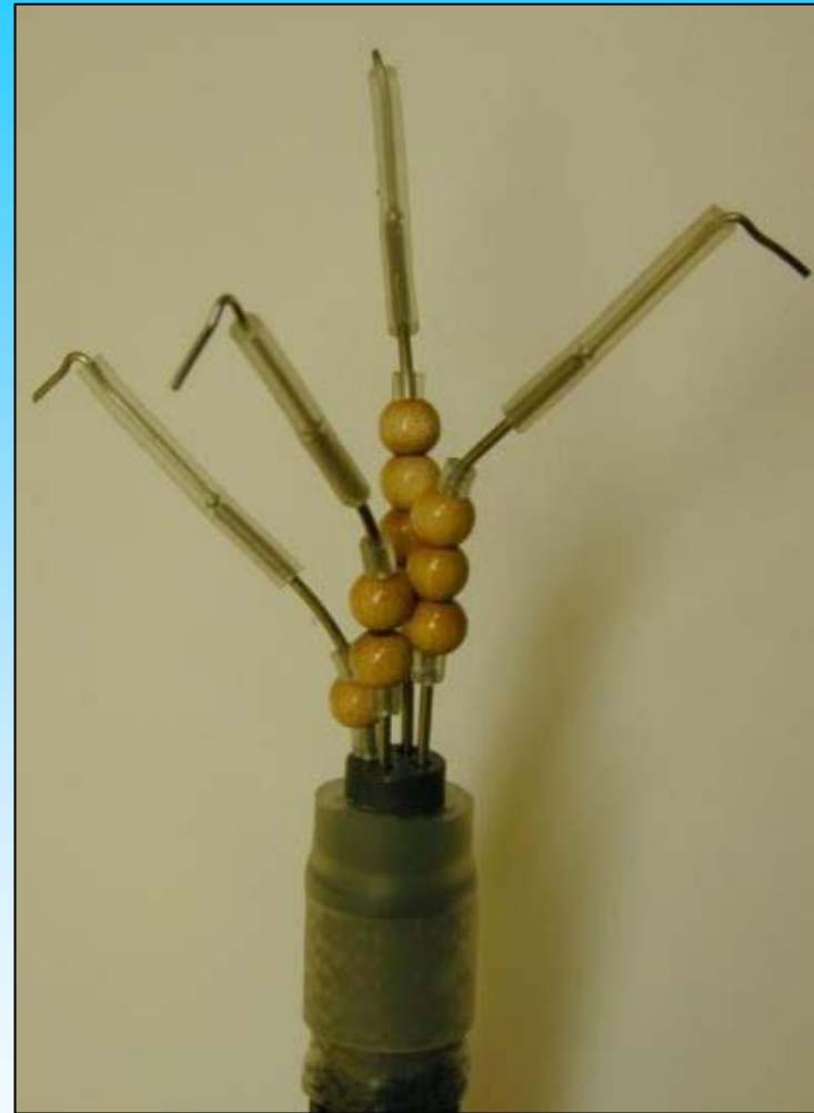
Top end of GASSYS installation showing the stainless steel microtubes for taking samples from four distinct collection chambers.
