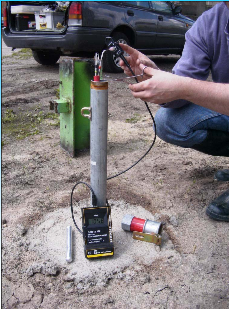
Measurement of gas pressure within sampled GASSYS chamber
