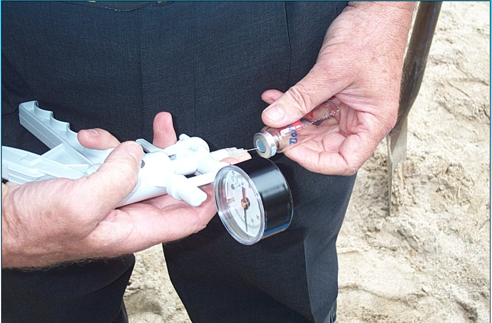
Evacuation of air from a headspace vial.
