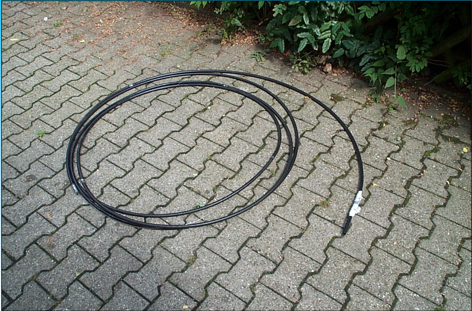
GASSYS hose with two semipermeable collection chambers prepared for installation.
