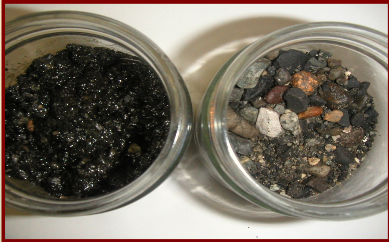
Pre and Post Ivey-sol Treatment Effective Removal of Heavy-end Hydrocarbons.
